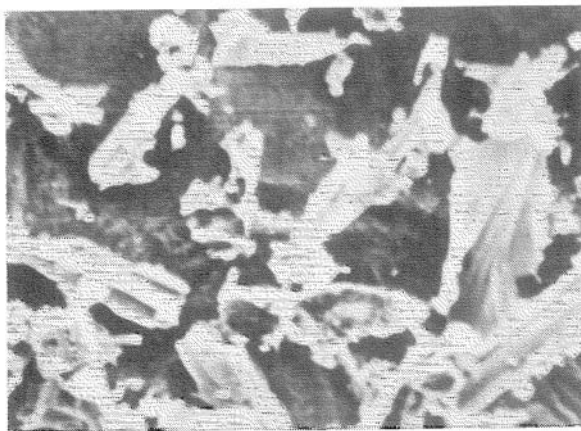
FIG. 1 SEM photograph of bagasse fly ash at 320 \times .
